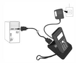
Warning: When both RS-232 and USB cables are connected between the cradle and host computer, the USB interface takes priority for data transmission and the RS-232 communication is automatically disabled.
