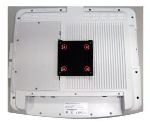
2. Mount M1920 onto desktop-stand through the conversion bracket covered in accessory kit as well.
