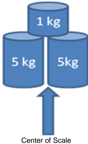
Figure 4-3 Weight Calibration Configuration for Kilograms
