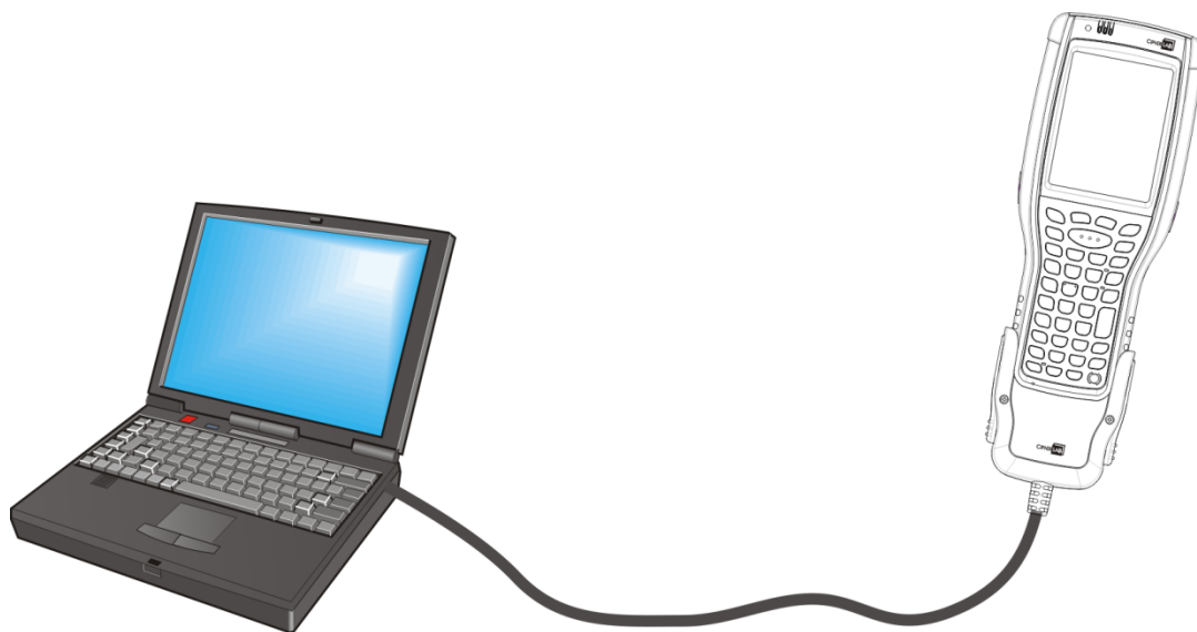
Figure 11: Direct Data Communication Using Snap-on Cable
