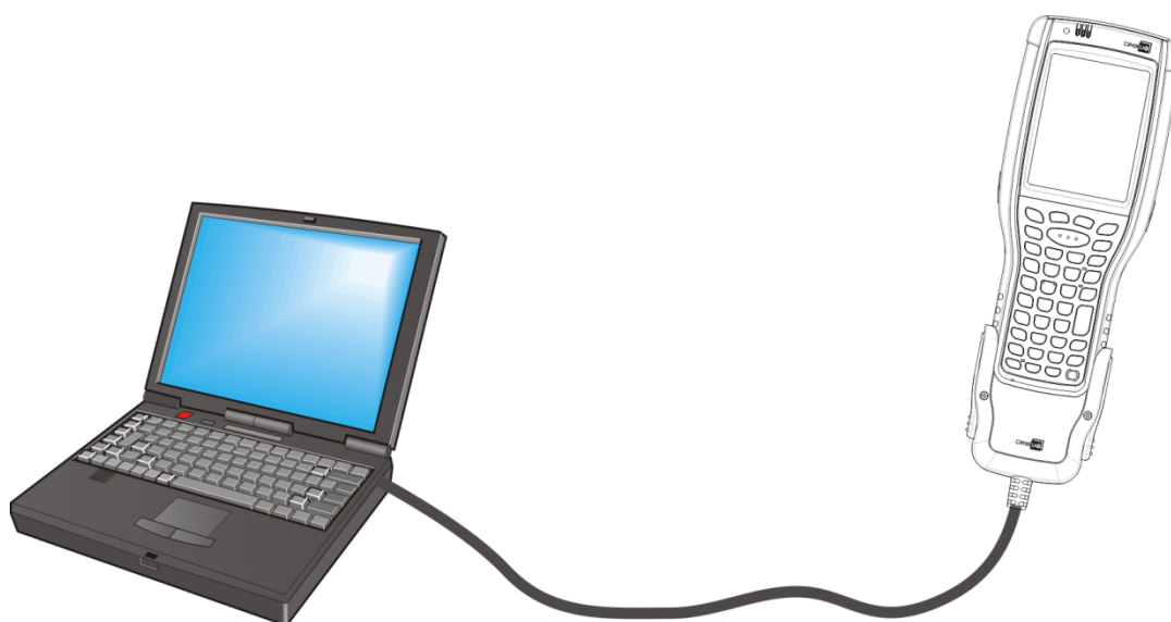
Figure 11: Direct Data Communication Using Snap-on Cable
