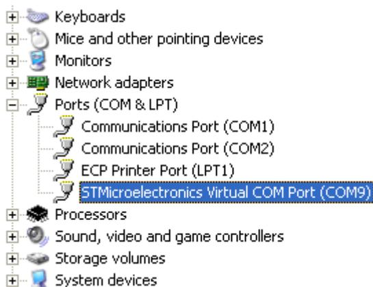
The available COM Port number should be at COM1~COM9. If the allocated COM Port number is greater than 9, change it within 9. Right-click on "STMicroelectronics Virtual COM Port (COM)". Click: Properties -> Port Settings -> Advanced -> COM Port Number. Select a COM Port Number within 9.
