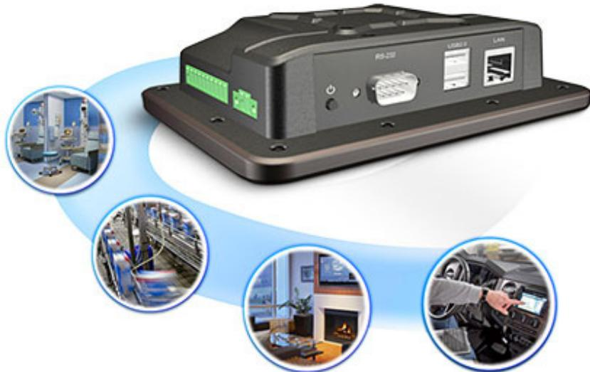
So what does such a miraculous box look like, and what's in it? It's small, just 5.9 x 4.3 inches, and only weighs 13 ounces or so. It technically *is* a little panel PC, but one that runs Android 5.1 and has a very nice 5-inch screen with capacitive multi-touch. And just like in any modern smartphone, flush glass extends well beyond the perimeter of the LCD screen, so that your fingers can easily operate it without bopping into a frame.
